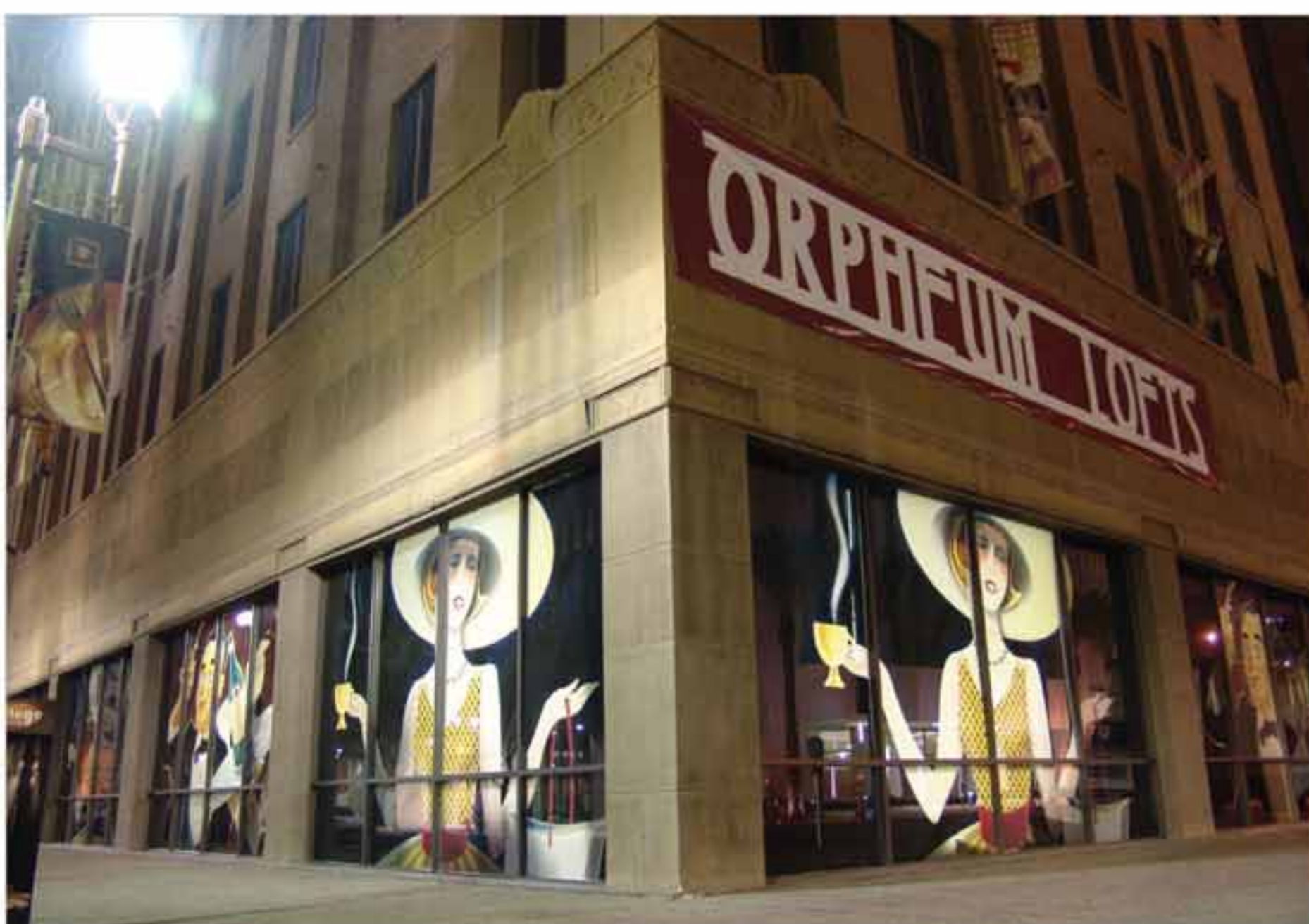
Another example of lifestyle prints, these vacancy graphics produced by Bluemedia during construction of the Orpheum Lofts condo project in downtown Phoenix, were printed on translucent backlit film and double stick taped to the inside of the windows.
